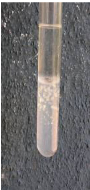
Fig. 1 Prismatic transparent, semitransparent, and well-defined crystals of calcium cadmium tartrate In gel of density 1.04 \text{ g/cm}^3
